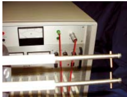
Capacitive spark generator for use with a 20 litre sphere apparatus.
