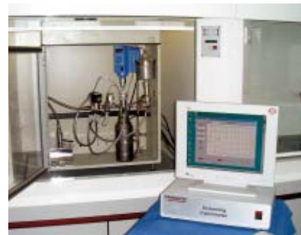
Waste Stream Screening Calorimeter
