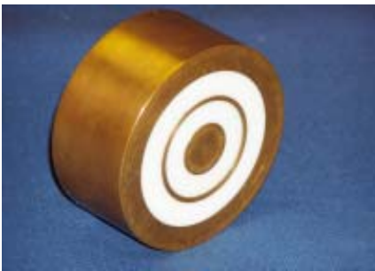
Concentric rings test electrode - in compliance with standards listed above.
