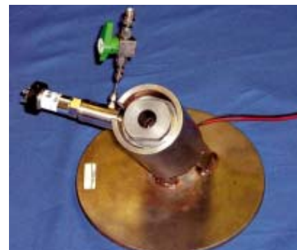
Time Pressure Test Vessel (Can also be used for oxidising liquids tests - see page 6.)
