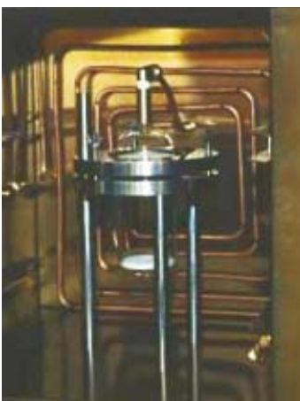
Internal view of oven - Aerated Cell and mount. Shows sample vessel and mounting stand together with air pre-heating pipework. For the Diffusion Cell test, the vessel lid is detached from the main vessel body to allow natural air diffusion.
