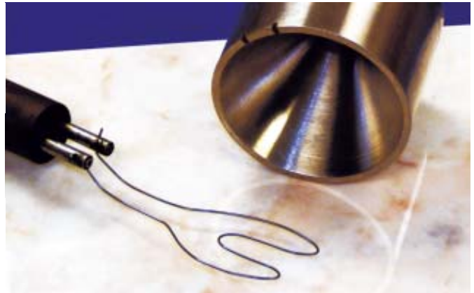
Oxidising solids apparatus - shows sample loading chamber and hot coil.
