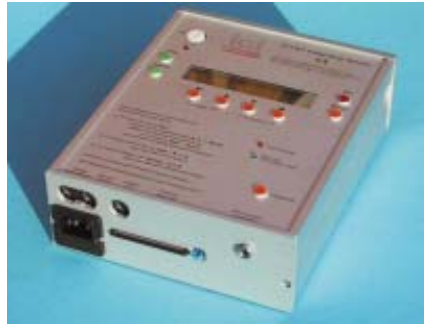
Charge relaxation time measurement apparatus (JCI 155v5) for powders, textiles and liquids.
