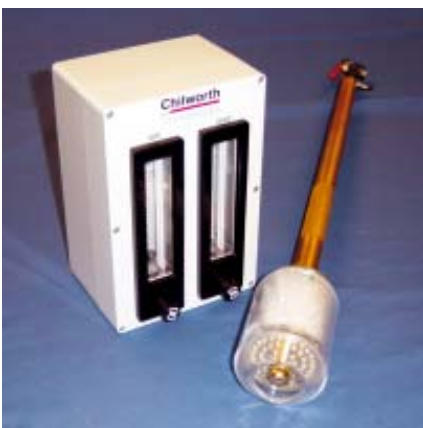
Gas probe & mixing equipment for estimation of discharge energy drawn from surfaces. Spark ignition calibration unit not shown (optional extra).
