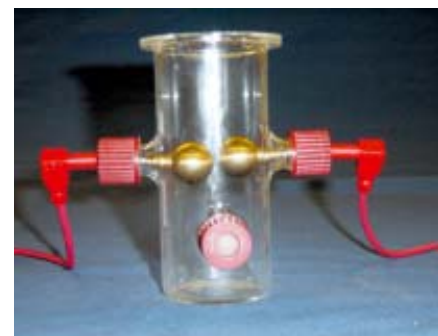
MIE of Gases/Vapours (Vapour test vessel and electrode assembly shown.)
