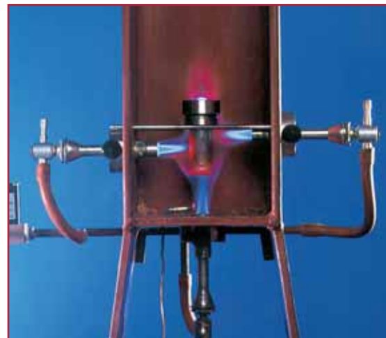
Koenen Tube Explosivity Test Apparatus
